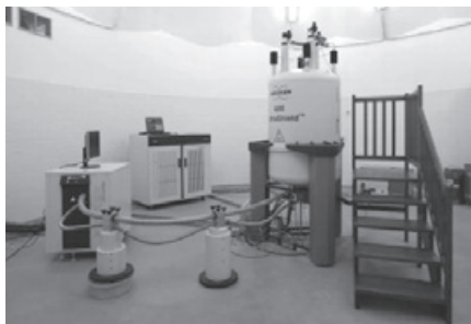
600 MHz NMR spektrometr Bruker AVANCE.
